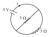
In the final diagram, we can write equivalent resistance across the battery as  $\ 2.5\ \varOmega.$
