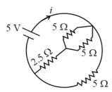
As in this case,  $5~\Omega~\&~5~\Omega$  are in parallel hence, their combined resistance value will be  $2.5~\Omega$ . Now, this  $2.5~\Omega$  with existing  $2.5~\Omega$  are in series and hence can be combined to write  $5~\Omega$ .
