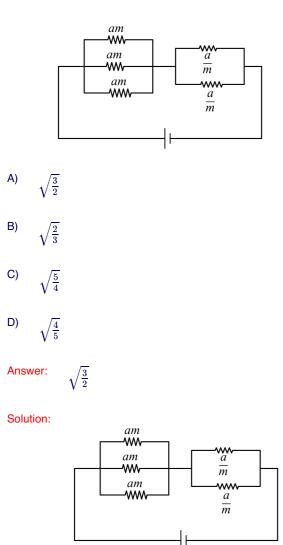
Left part of the resistors are connected in parallel, hence  $R_1 = \frac{am}{3}$ . Similarly for the right part of the resistors we can write,  $R_2 = \frac{a}{3m}$ .
