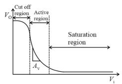
The saturation zone and cut-off area are known as the transistor switch's working regions. This implies that, by switching between its "top-off" (saturation) and "absolute OFF," the transistor is used as a switch.
