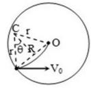
$$egin{aligned} r &= rac{mV_0}{qB} \ R &= 2r\,\sin heta \ \Rightarrow R &= rac{2mV_0}{qB} \!\sin heta \ \Rightarrow V_0 &= rac{qBR}{2m\sin heta} \end{aligned}$$
