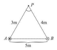
Magnetic field due to first wire (A) is  $B_1=\frac{\mu_0\times I}{2\pi\times 3}$ Magnetic field due to second wire (B) is  $B_2=\frac{\mu_0\times I}{2\pi\times 4}$ Net magnitude of magnetic field  $B=\sqrt{B_1^2+B_2^2}$
