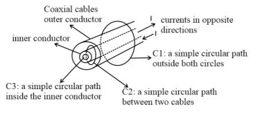
At outside the cable for loop  $C_1$  and inside the cable for loop  $C_3$ , the enclosed current is given as,
