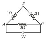
Here, two resistance of  $1~\Omega$  and  $2~\Omega$  are in series, which is equivalent to  $3~\Omega$  which is in parallel with  $3~\Omega$  resistance. Therefore, the effective resistance is,
