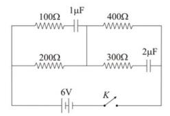
In steady state, arm having capacitors does not flow current. So, we can neglect them.  $\therefore$  The given circuit reduces to
