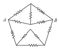
The upper part is the example of a Wheatstone bridge. It means the resistance at the middle of the upper part is shunted.
