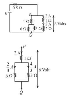
As in the above branch potential across PQ is 6 V and equivalent resistance is  $3 \Omega$ , therefore current in this branch should be 2 A. Therefore voltage across  $6 \Omega$  is 4 V and hence current in it is  $\frac{2}{3} A$ .
