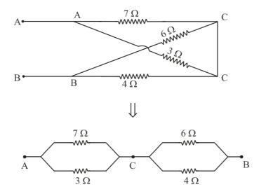
Now, we can see that 7  $\Omega$  and 3  $\Omega$  are in parallel between A and C and 6  $\Omega$  and 4  $\Omega$  are in parallel between C and B.
