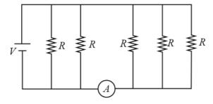
Total resistance of five identical resistors in parallel,
