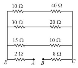
Hence, the resistance  $R_{CE}$  between CE can be calculated by using parallel combination of resistances after combining the resistances in series in each branch.
