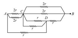
We can see that between A & C, the terminal 2r and 2r resistances are in parallel combination, and we can calculate using the following relation  $\left(R_{eq} = \frac{R_1 \times R_2}{R_1 + R_2}\right)$ .
