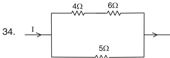
In the above circuit, the heat produced in  $5\Omega$  resistance is 10 calories per second. The heat produced in  $4\Omega$  resistance is
