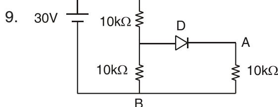
In above circuit, potential difference between A and B is
