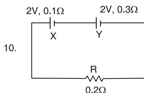
The internal resistance of two cells shown are  $0.1\ \Omega$  and  $0.3\ \Omega$ . If  $R = 0.2\ \Omega$ , the potential difference across the cell
