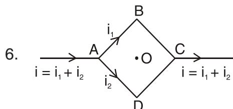
Above circuit shows a square loop ABCD with edge length  $a$ . The resistance of the wire ABC is  $r$  and that of ADC is  $2r$ . The value of magnetic field at the centre O of the loop assuming uniform wire is
