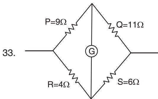
How much resistance must be put in parallel to the resistance S to balance the above bridge ?
