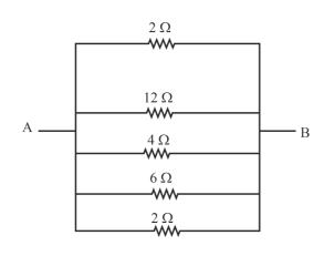
Since all the resistors of the redrawn circuit are in parallel,
