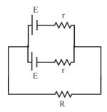
When cells are in parallel combination, as shown above, the equivalent EMF
