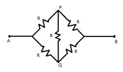
Since the circuit is in balanced wheatstone configuration, the capacitor and the resistor connected across points P and Q can be omitted. Now, the circuit has two arms having two resistors connected in series.
