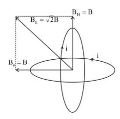
Here,  $\mathit{B}_{V},\ \mathit{B}_{H}$  are the magnetic field due to the vertical and the horizontal loop, which by magnitude are equal.
