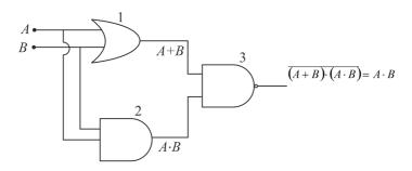
As can be seen from the above diagram, gate 1 is an OR gate, gate 2 is an AND gate and gate 3 is a NAND gate.
