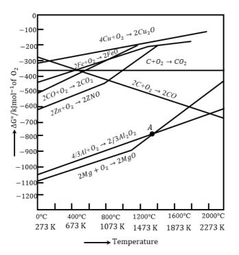
From the graph each metal oxide line started to move upward towards positive value of  $\Delta G$ . The metal oxide formation is not possible if it is unstable. So every metal oxide is unstable at a certain point. From the diagram it is clear that both the statements are correct.
