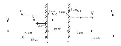
Considering the image formation started at mirror A at first, the first image is formed at position  $I_1$  behind it. Considering  $I_1$  as object and reflection at mirror B, an image is formed at  $I_1$ ' behind mirror B. Similarly, the next image is formed at  $I_2$  behind mirror A.
