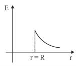
Solution: For a conducting spherical shell, the total charge resides on its surface.
