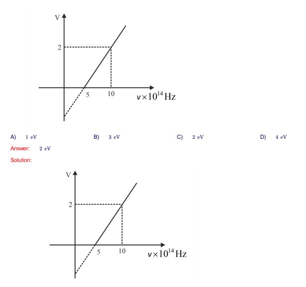
The interception of the stopping potential versus frequency curve indicates the ratio of the stopping potential of the material to the charge of electron.
