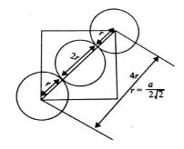
The relationship between radius of lattice(r), edge length(a) of an FCC unit cell is  ${
