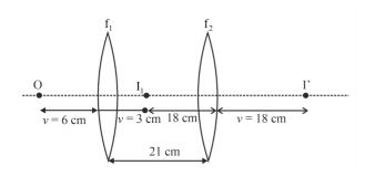
Considering the left lens at first, the image distance (v) can be calculated as follows-
